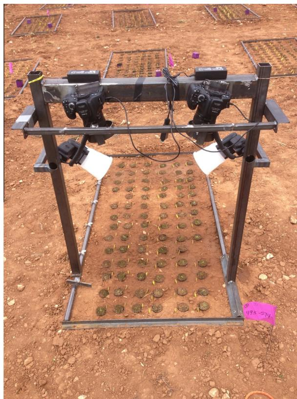
**Fig. 4.** Field imaging platform. The ground-level field imaging setup. Two Canon DSLR cameras were mounted with an angle. Two flashes with diffusers were mounted on the side bars for creating a uniform illumination condition.
