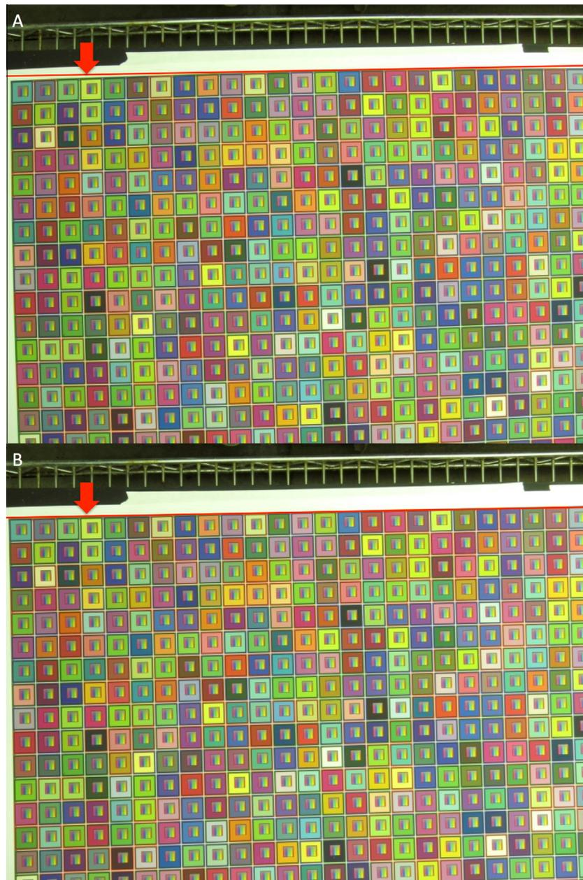
**Fig. 8.** Image optical distortion correction. (A) The image before the image optical distortion correction. The red reference line on the top shows the curvature of the edge of the color grid. (B) The image after the image optical distortion correction. The edge of the color grid shows straight comparing the red reference line. (For interpretation of the references to colour in this figure legend, the reader is referred to the web version of this article.)
