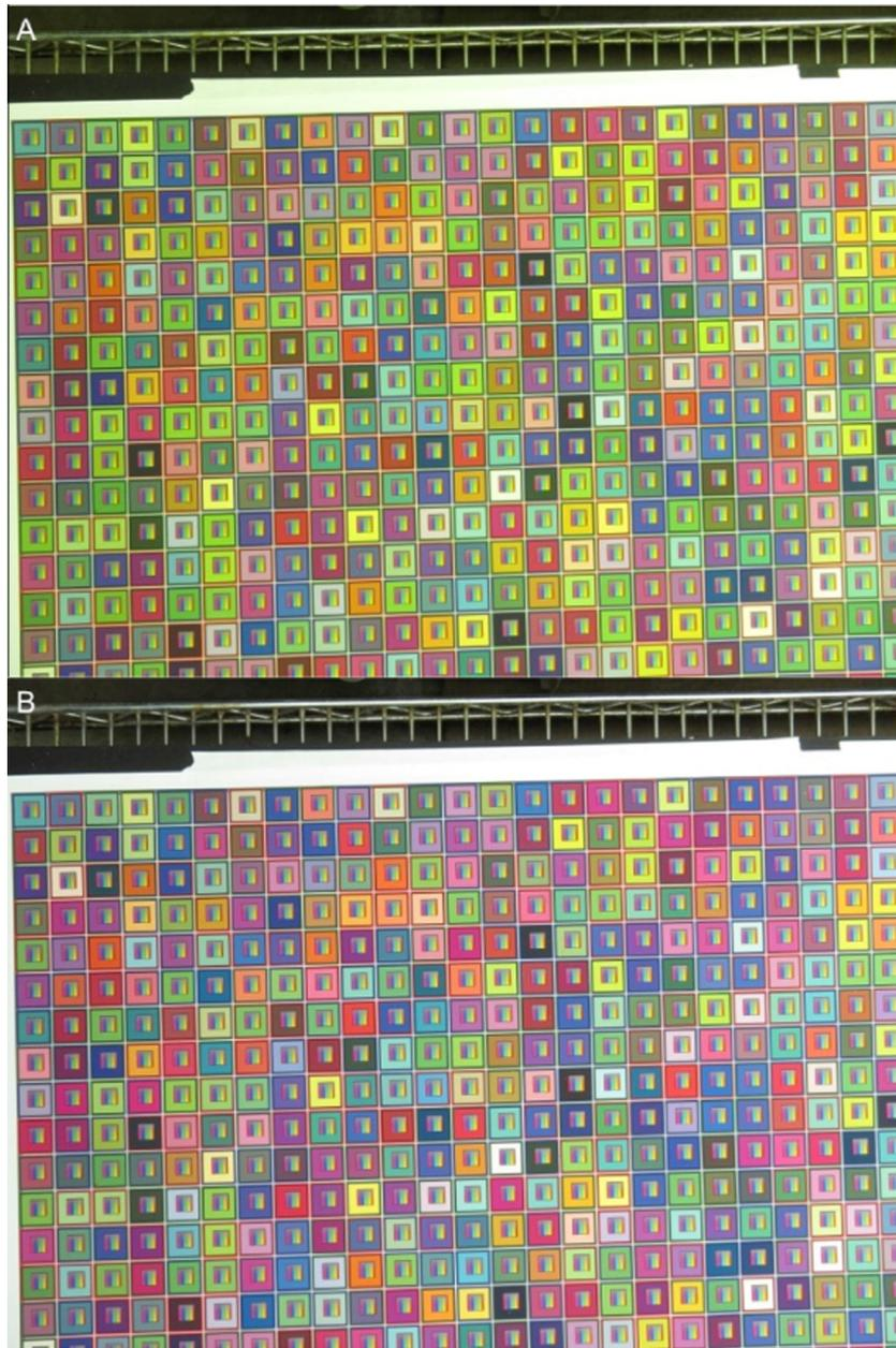
**Fig. 9.** Image color correction. (A) The image before the image color correction. The green tone of the image was due to shelf illumination. (B) The image after the color correction shows that the green tone was removed. (For interpretation of the references to colour in this figure legend, the reader is referred to the web version of this article.)
